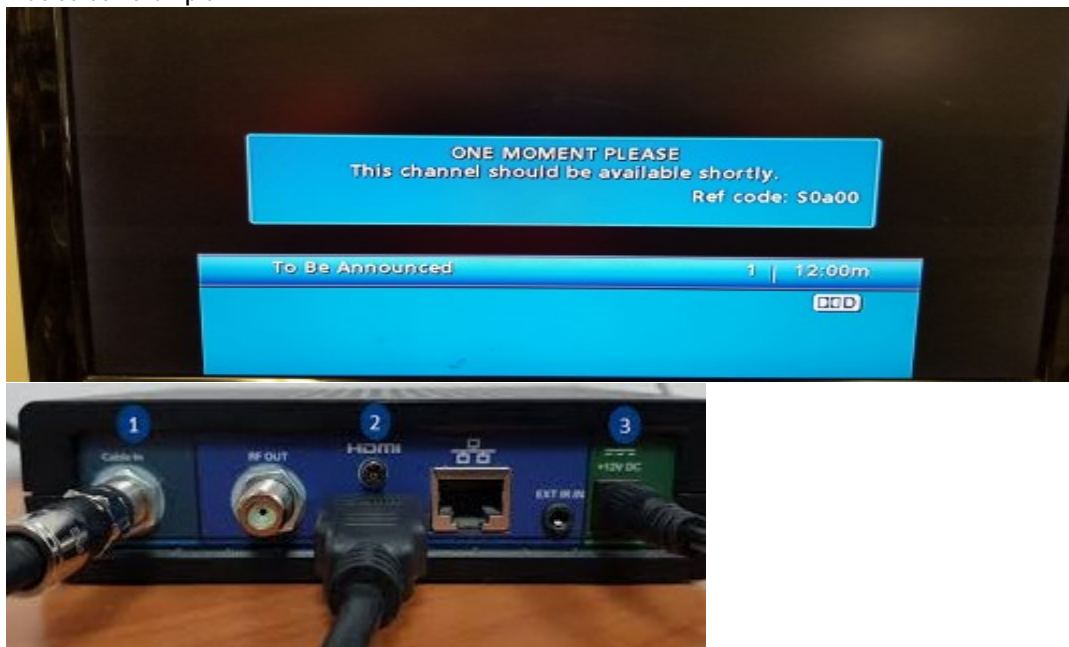
1. Coaxial connection from wall 2. video source connection 3. connection for power
